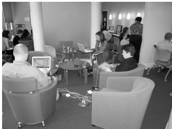
Outlets in the floor allow increase ubiquitous power and connections for mobile equipment
